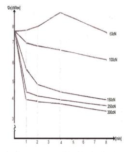
Fig. 2:Effect of time and load level in the elastic stress
