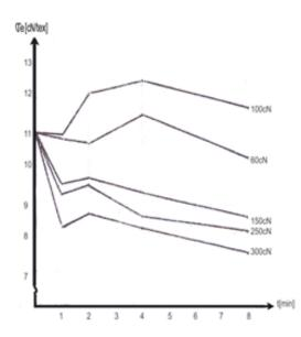
Fig. 4:Effect of time and load level in the yield stress
